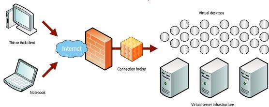
which shares a slice of a Windows Server operating system and applications to each end user, a virtual desktop is its own unique environment, usually loaded with a Windows Vista/Windows 7/XP operating system and applications that can be locked down or left open to end-user customization.
