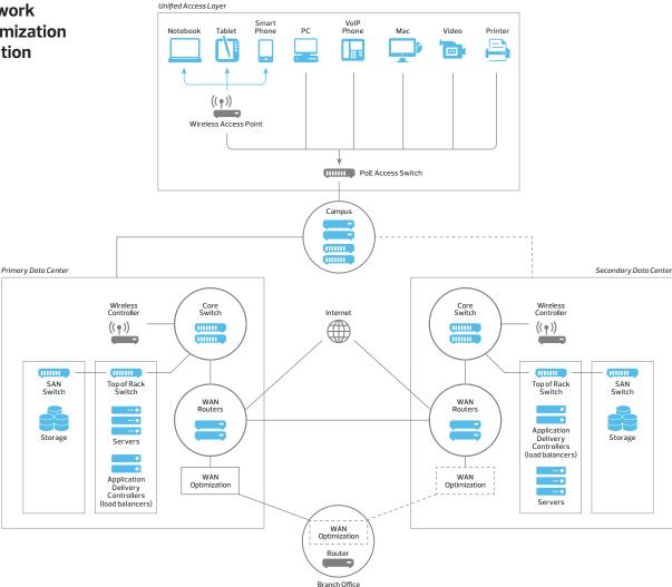
These extensions unlock distributed clustering and other capabilities at the web, application and database layers. IPbased OTV can also deliver value inside the data center, where it improves mobility by working with Layer 3 interconnects, which effectively segment the network.
